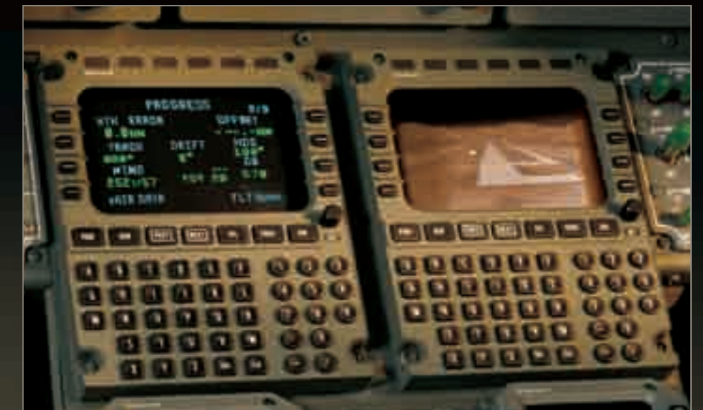
Enhanced Vision System (EVS). In flight and on the ground, infrared sensors enhance the situational awareness required to navigate in rain, snow, haze, smoke and total darkness.
